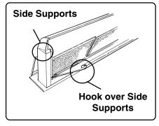
Hook the top of the front intake panel over the side supports at the top of the ventilator.
